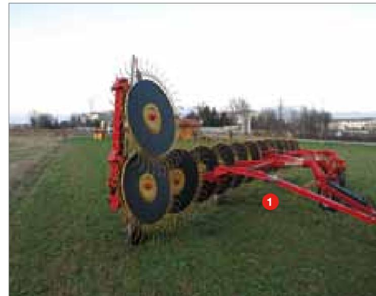
For transfers a hydraulic device allows the first two front finger wheels to be raised, reducing the rake length and making the machine more compact.
