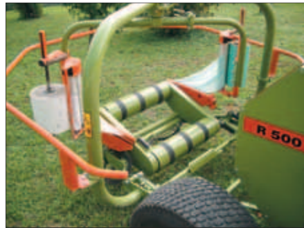
Hydraulic arm transferring the bale from the roundbaler to the wrapper.
