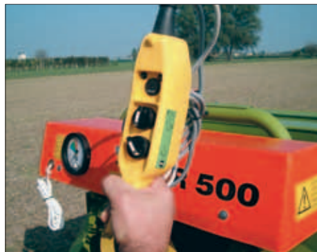
The electric push button panel allows to perform all the functions directly from the tractor (A= back door open-close, B= pick-up raising-lowering). In addition, on the push button panel there is the acoustic signal which warns when the bale is ready. The integrated bale counter keeps the record of the bale made.
