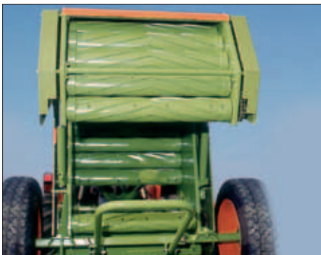
Aluminium rollers bale chamber specially designed to guarantee a consistent and perfect rotation of the bale.
