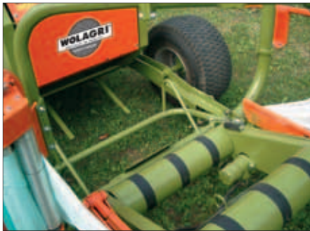
Wrapping system with 2 rotating arms and 2 stretchers ensuring a quick and effective wrapping. Film is cut by 2 hydraulic knives.
