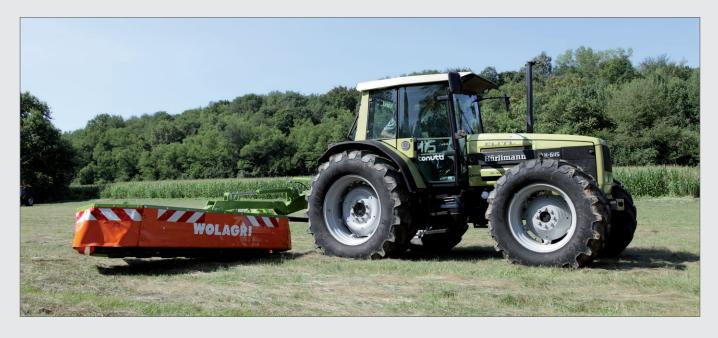
The POLARIS machines all have a "Nonstop" safety release with which it is possible contact of the mowing unit with the ground for positioning it vertically. to continue to cut without having to stop the tractor unit and without reversing after the grassy layer being damaged. finding an obstacle. The re-coupling is automatic, without operator intervention or hydraulic means, increasing machine lifespan.
