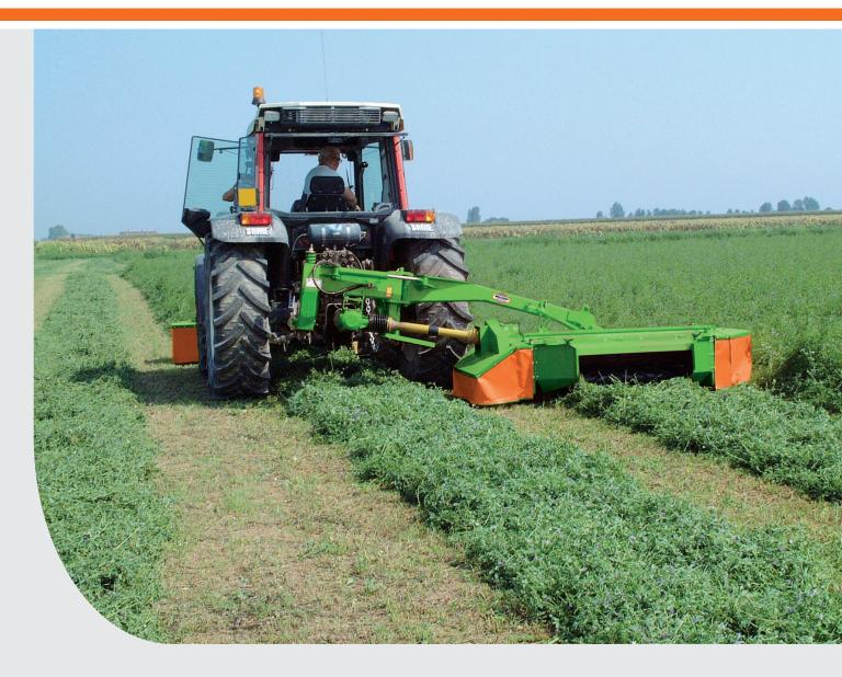
• Very thick cover (5 mm) with integral reinforcement. This cancels out flexing of the cutting group so as to avoid twisting of the moving parts.
