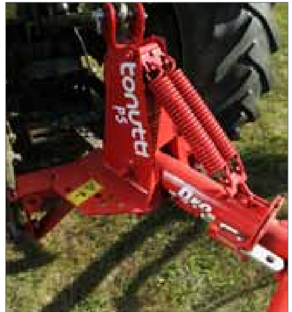
Three-point attachment with double spring suspension
