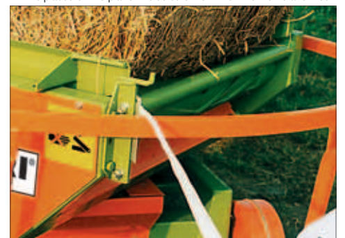
A knife placed on the platform side cuts the film on the first rotation tour.
