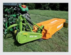
A compensating spring provides excellent adjustment to the weight of the mower reducing the pressure on the ground to ensure a perfect cut without damaging the grassy scalp.
